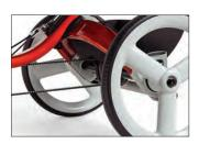
**Carbon fiber drive belt** The drive belt will not rust or stretch, and will last at least five times longer than a bicycle chain.
