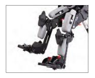
Advanced legs have independent leg length, hip angle and knee angle adjustments.
